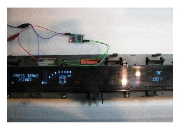
Simple connection -4 wires only: **CAN Low, CAN High,** +12v, **GND**. After power on emulator turns on dashboard. If everything is connected correctly and there are no CAN faults **RED LED** on emulator board is blinking.
